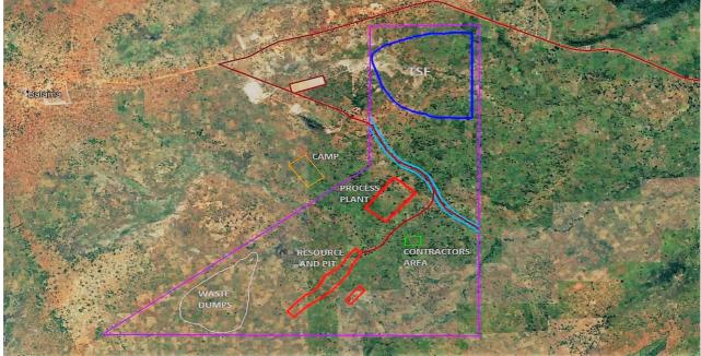
Figure. Mine layout and design showing location of the Mining Pits and waste dumps and mine infrastructure locations for plant ore stockpile, tailings storage facility, water storage dam and permanent camp
