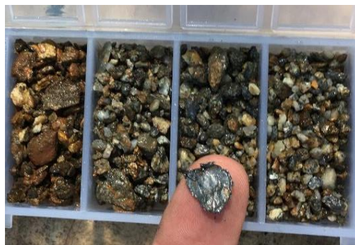
Figure 13: Example of the graphite mineralization observed in follow up drilling around significant intercept form EL258A. Approximate width of flake is 10mm.
